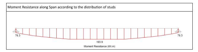
Critical Total Moment from Analysis  $M_c = 268.7 \text{ kN.m} \{ \text{Comb: ULS 2 @ } 4.0 \text{ m } \}$
